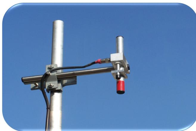
■ UHF NARROW BAND DIPOLE ANTENNA
